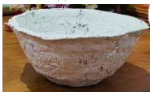
(a) Biopack Made from Recycled Paper
