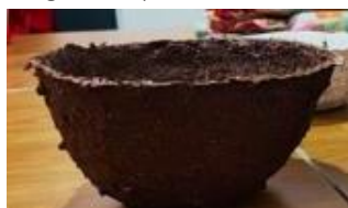
(b) Biopack Made from Dried Leaves
