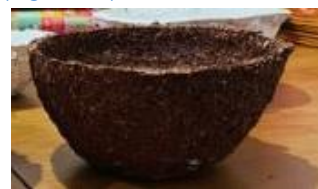
(c) Biopack: A Blend of Recycled Paper and Dried Leaves
